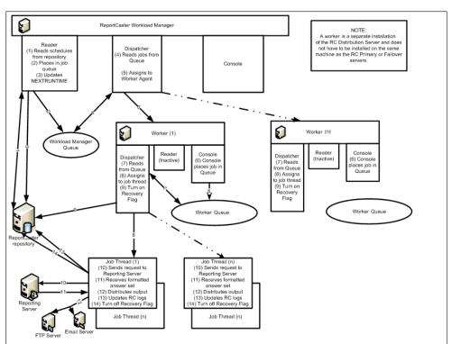
The following diagram illustrates the processing and relationship between the Workload Manager and its Workers.
