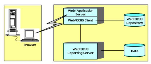
□ **Distributed Configuration.** In a distributed configuration, the WebFOCUS Client is installed on your web server, but the WebFOCUS Reporting Server and source data are on a different machine.
