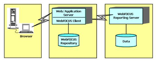
Multiple Data Source Configuration. If you have source data on several different machines, WebFOCUS can integrate that data into one reporting environment. To allow this, instances of the WebFOCUS Reporting Server should be installed on machines with access to your source data. WebFOCUS technology provides the data access and format conversion functionality. For more information on integrating data from multiple machines and platforms, refer to the server documentation.
